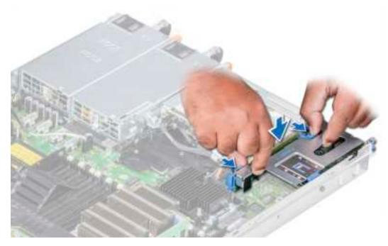
Figure 55. Installing the expansion riser 1B
