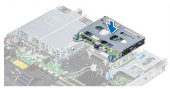
Figure 96. Installing the rear drive cage
