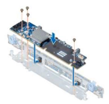
Figure 94. Installing the SAS expander card
