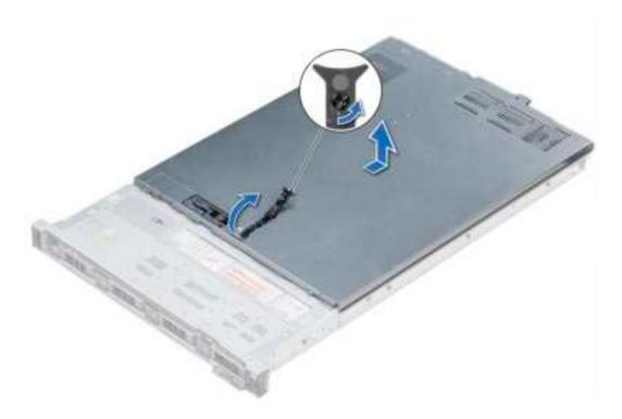
Figure 21. Removing the system cover
