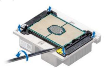
Figure 44. Loosening the processor bracket
