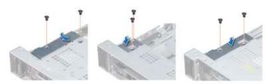
Figure 115. Installing the cable cover
