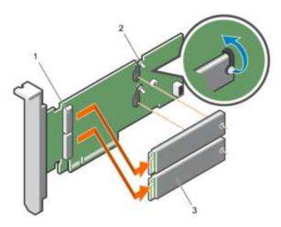
Figure 67. Removing the M.2 SSD module
