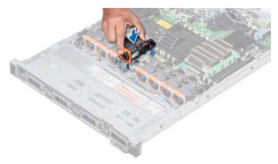
Figure 37. Installing the cooling fan
