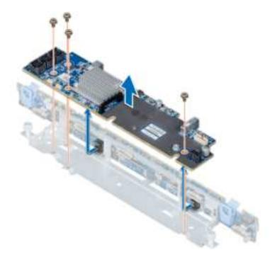
Figure 93. Removing the SAS expander card
