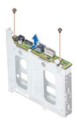
Figure 84. Removing the 2.5 inch drive rear backplane
