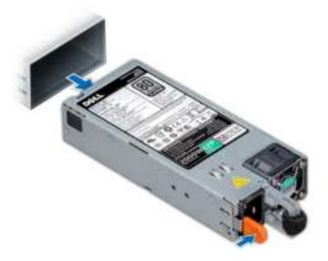
Figure 107. Removing a power supply unit
