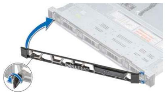
Figure 20. Installing the optional front bezel with the LCD panel
