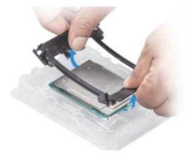
Figure 45. Removing the processor bracket
