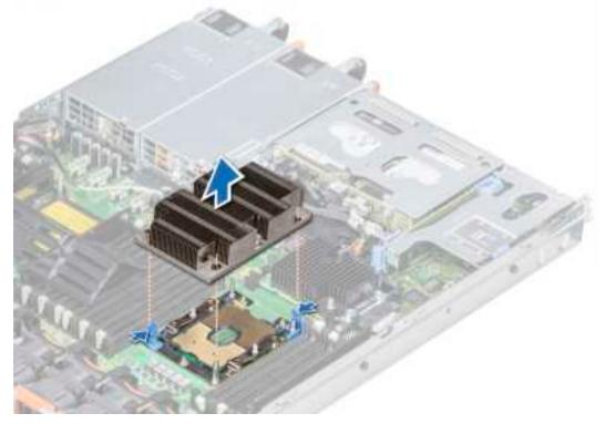
Figure 43. Removing the processor and heat sink module
