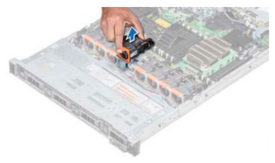
Figure 36. Removing the cooling fan
