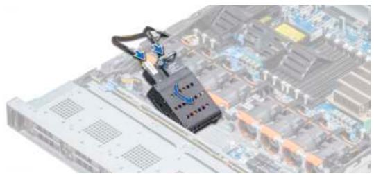
Figure 42. Installing the NVDIMM-N battery
