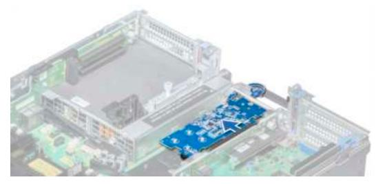
Figure 59. Removing the expansion card from expansion card riser 2B
