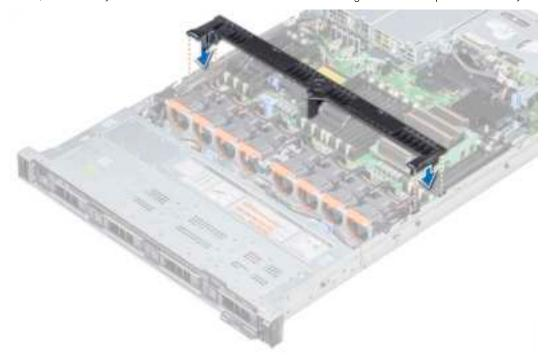
Figure 35. Installing the air shroud
