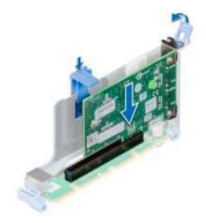
Figure 64. Installing an expansion card into the expansion riser 1B
