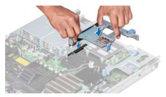
Figure 57. Installing the expansion riser 2B
