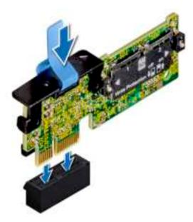
Figure 70. Installing optional IDSDM module
