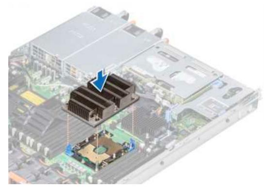
Figure 49. Installing a processor and heat sink module
