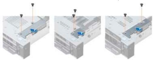
Figure 119. Installing the cable cover
