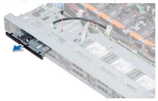
Figure 99. Removing the USB module
