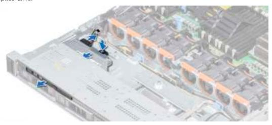
Figure 103. Removing optical drive
