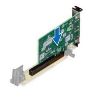
Figure 66. Installing an expansion card into the expansion riser 2A
