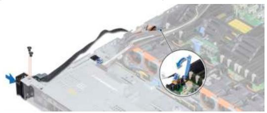
Figure 114. Installing the left control panel
