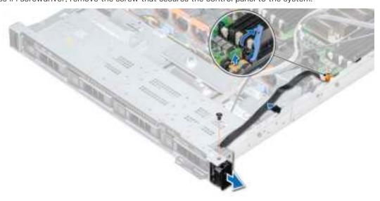
Figure 117. Removing right control panel
