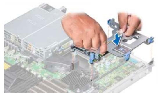
Figure 54. Installing the expansion riser 1A
