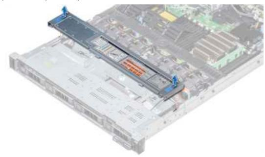
Figure 82. Removing the backplane cover
