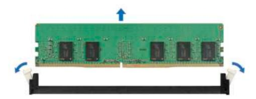
Figure 39. Removing a memory module
