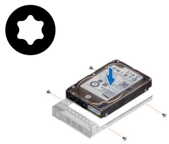
Figure 28. Installing a drive into the drive carrier
