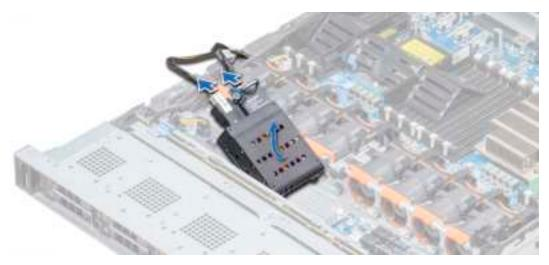
Figure 41. Removing the NVDIMM-N battery
