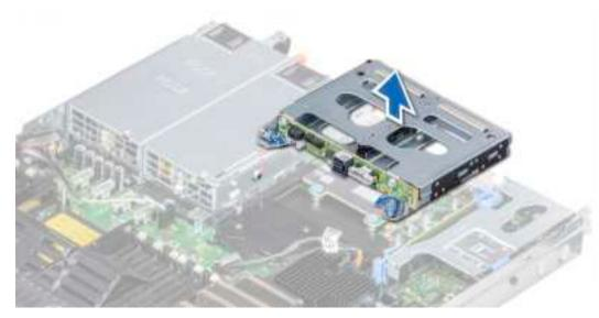
Figure 95. Removing the rear drive cage
