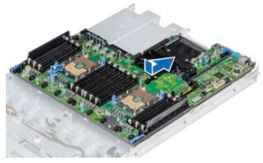
Figure 110. Installing the system board
