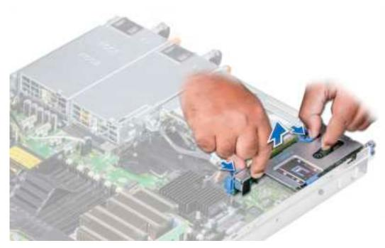
Figure 50. Removing the expansion riser 1B
