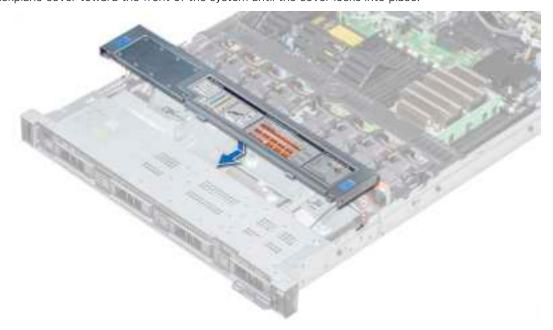
Figure 30. Installing the backplane cover
