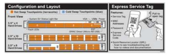
Figure 16. Configuration and layout and express service tag
