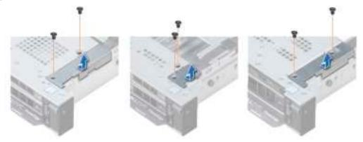
Figure 116. Removing the cable cover
