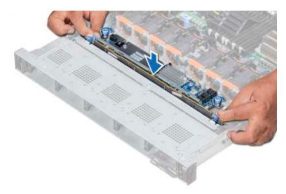
Figure 83. Installing the backplane
