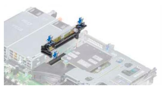
Figure 56. Installing the expansion riser 2A
