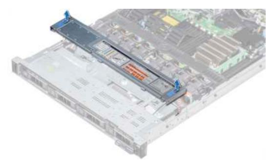
Figure 29. Removing the backplane cover
