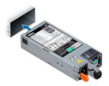
Figure 108. Installing a power supply unit
