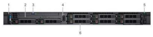
Figure 2. Front view of 8 x 2.5-inch drive system
