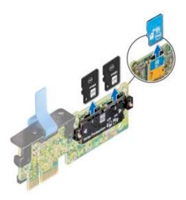
Figure 71. Removing the MicroSD card
