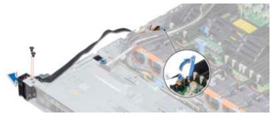
Figure 113. Removing left control panel
