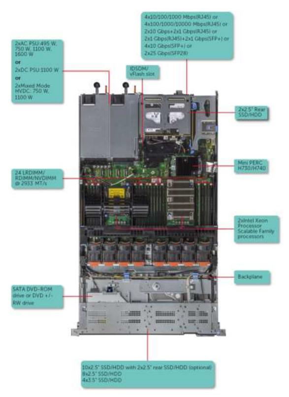
Figure 1. Supported configurations for PowerEdge R640
