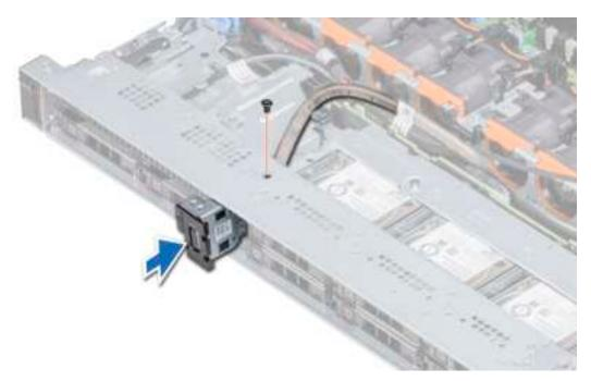
Figure 102. Installing the VGA module
