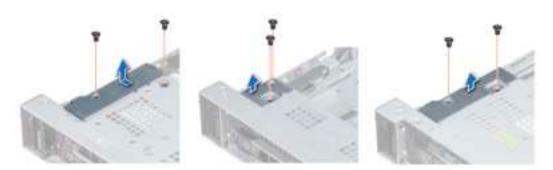
Figure 112. Removing the cable cover
