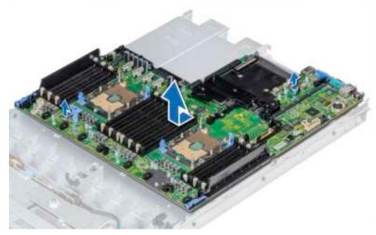
Figure 109. Removing the system board
