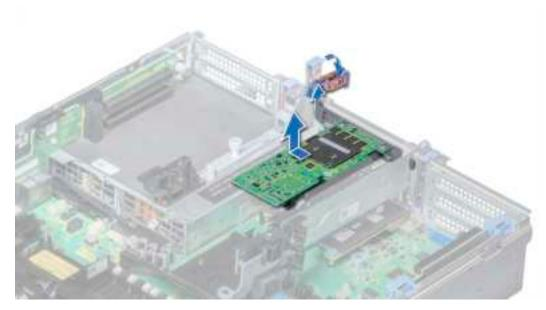
Figure 60. Removing the expansion card from expansion card riser 2
