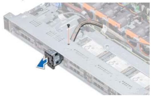
Figure 101. Removing the VGA module
