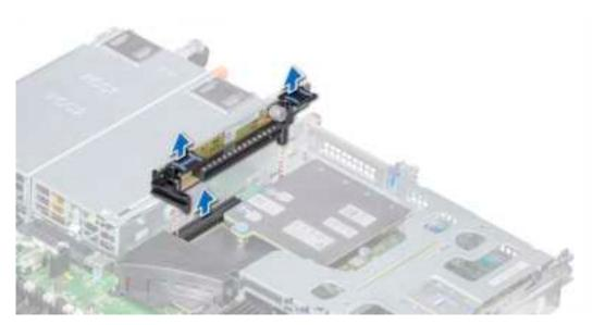
Figure 52. Removing the expansion riser 2A
