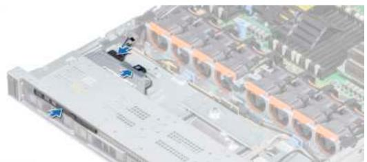
Figure 104. Installing the optical drive
