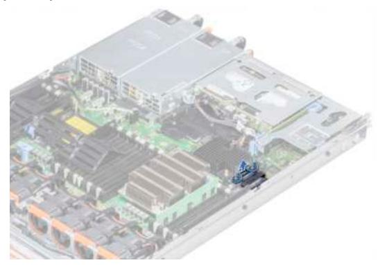
Figure 75. Removing the integrated storage controller cable
