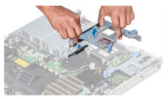
Figure 53. Removing the expansion riser 2B
