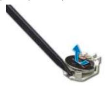
Figure 97. Removing the system battery
