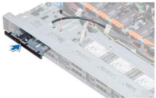
Figure 100. Installing the USB module
