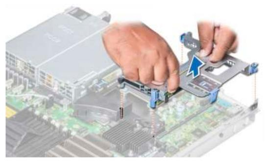
Figure 51. Removing the expansion riser 1A
