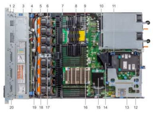
Figure 33. Inside the system - 3 PCIe expansion risers
