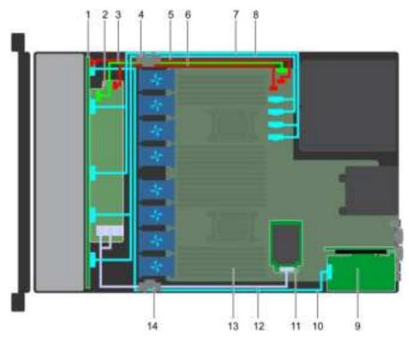
Figure 89. Cable routing - 10 x 2.5 drive backplane with NVMe
