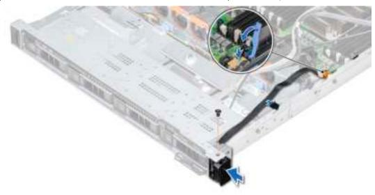
Figure 118. Installing the right control panel
